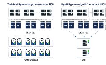
REVOLV is a hybrid hyperconverged solution, where only critical resources are stored in the vSAN cluster. By disaggregating video retention to a traditional SAN, REVOLV maintains high availability of critical resources, and VM mobility, without storing the video data itself with the cluster. This approach provides all the benefits of HCI while reducing hardware footprint, total cost of operations, and power requirements.
